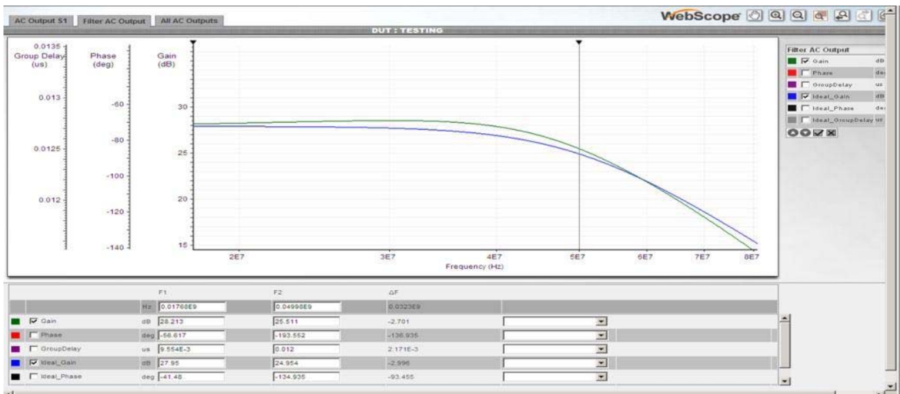
FIGURE 58. COMPARISON OF SIMULATED TO IDEAL GAIN RESPONSE
